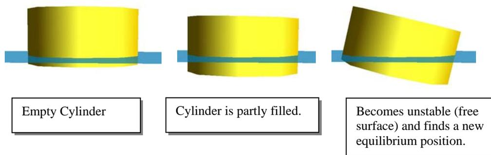
**Figure 2-21 Three stages of a floating cylinder.**
