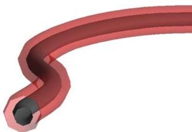
**Figure 2-23 Transversal connection between independent tubing- and riser elements.**
