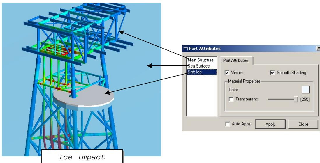
**Figure 2-14 Automatic Generated Parts.**
