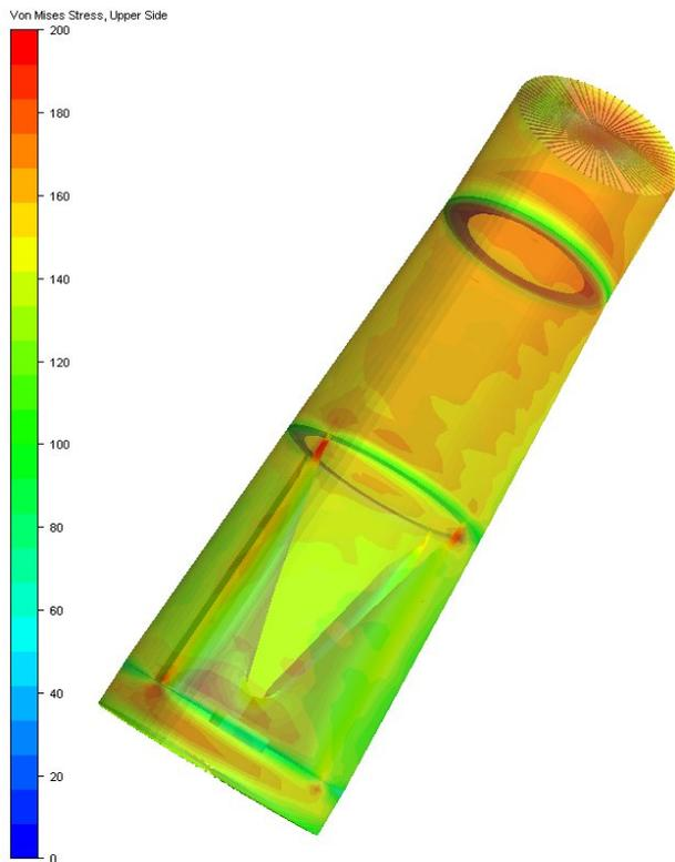
**Figure 2-16 Result Fringes (stress) applied on transparent structure.**
