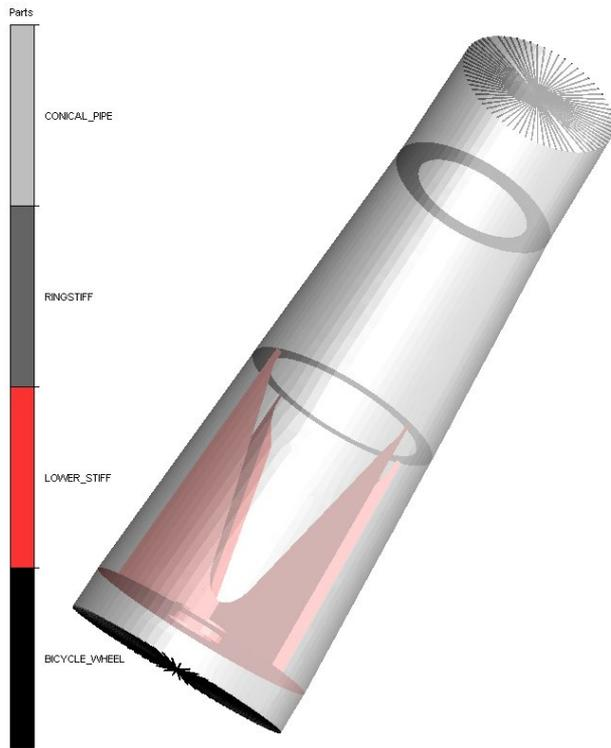
**Figure 2-15 Transparent Conical Shell showing inner stiffeners**
