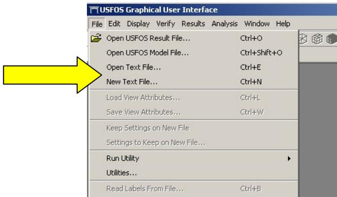
**Figure 2-17 Opening the editor (existing or new) general text file (\*.\*)**
