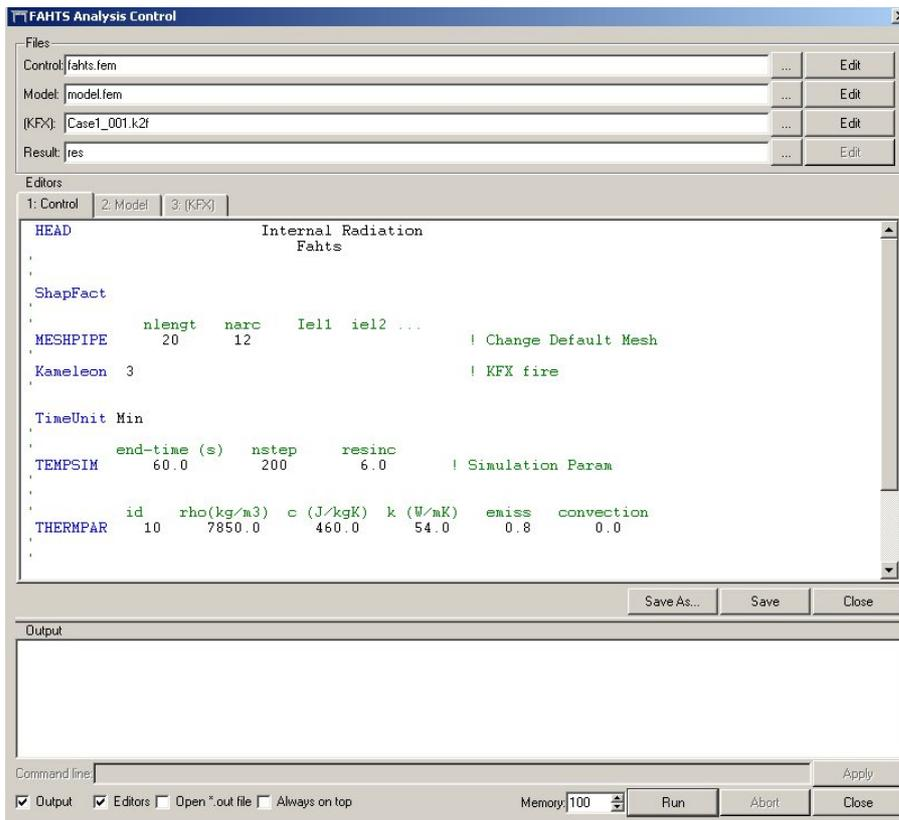
**Figure 2-6 Analysis Control for FAHTS .**
