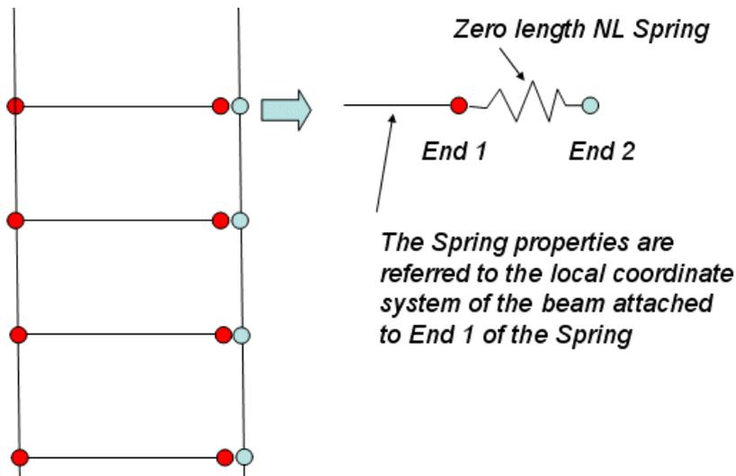
**Figure 2-22 Schematic description of Zero length 2 node springs.**
