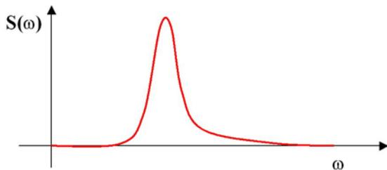
**Figure 2-19** Wave energy spectrum
