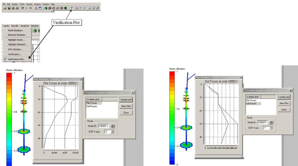
**Figure 2-14 Extended Plot Option for Pile/Soil**
