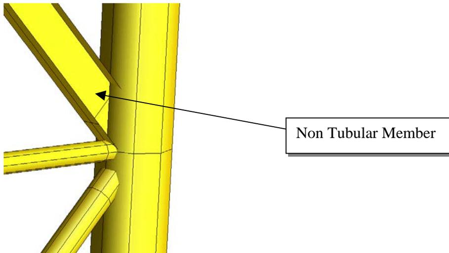
**Figure 2-12 Non Tubular Brace among tubular to check.**
