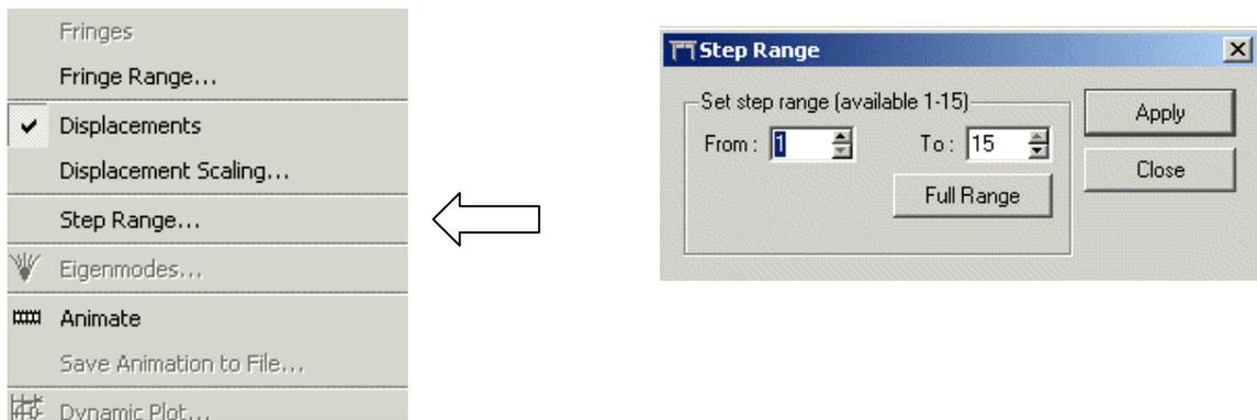
**Figure 2-2 Limit Result steps. Step Range is found in the Results menu**
