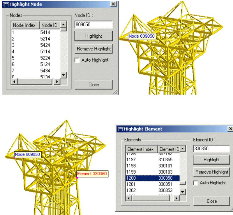
**Figure 2-5 Highlight Elements and Nodes**
