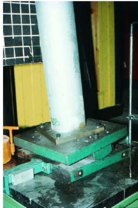
Figure 12-9 Support arrangement for the columns
