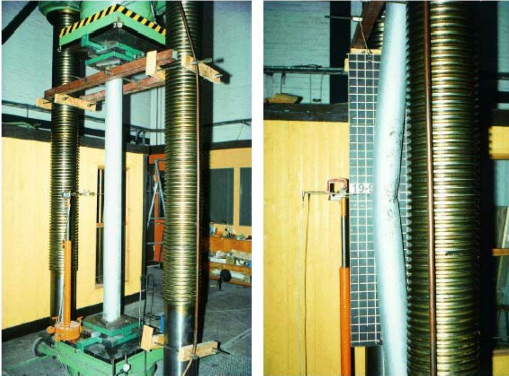
Figure 12-8 Test set-up and column in post-buckled condition
