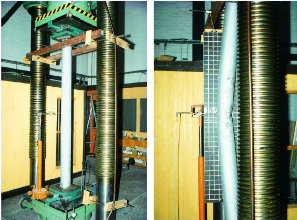
Figure 12-8 Test set-up and column in post-buckled condition
