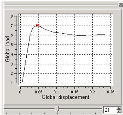
The main plot window will show the default plot for the analysis. Once a model is opened, you can set the load step from this plot window. There are several ways to set the load step. Either by clicking on the point in the plot you want to go to, by dragging the bottom slider, or by using the spin box in the lower right corner. Read more about plots in the “Plots” chapter.
