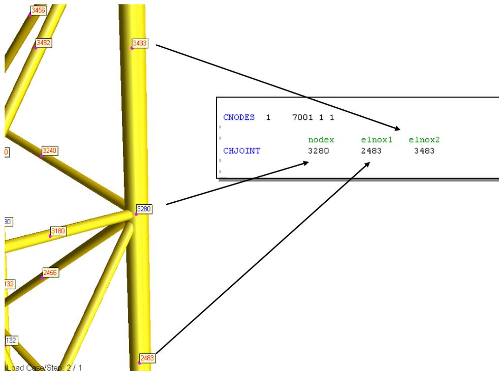
**Figure 3.3-15** Selecting node and element ID's by pointing on the 3D image.
