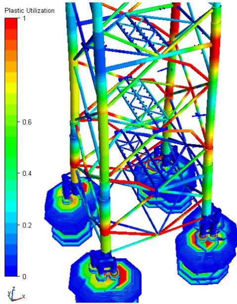
**Figure 3.4-5 Plastic Utilization of structure and pile/soil foundation**
