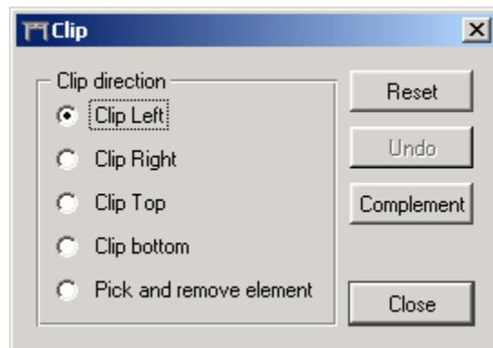
The “Complement” button shows all parts that are clipped. When you press the “Complement” button, the text on it will change to “Clipped”. If you press the button now, it will show the original clipped model.
