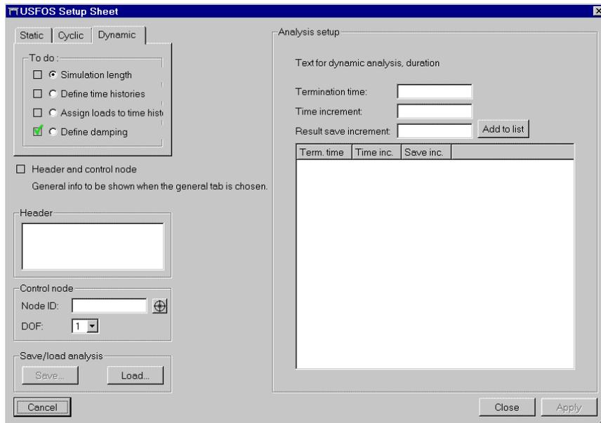
**Figure 3.3-6 Setup sheet for dynamic analysis. Empty**
