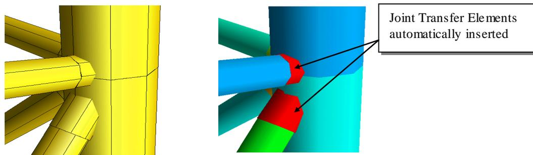
**Figure 3.3-16** USFOS analysis with Joint Resistance Limitation applied.
