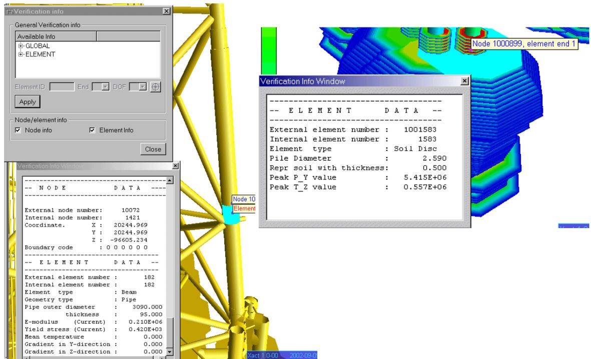
**Figure 3.4-3 Print of Node- and Element Information.**
