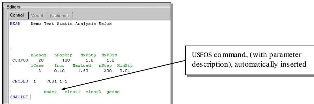
**Figure 3.3-14 Automatic inserting of the CHJOINT Command in the USFOS editor.**
