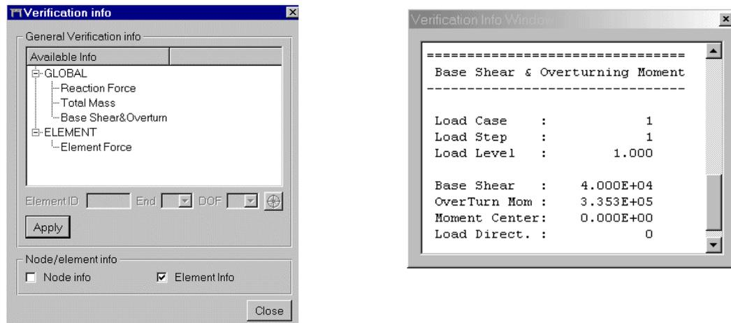
Figure 3.4-10 Verification Info and print of Base Shear etc for a given load step.
