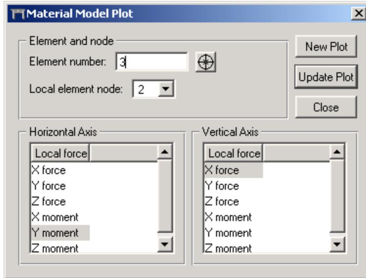
The material Plot dialog lets you create a Material Model plot. You can type the Element ID and Element End you want the plot to represent. As in all dialogs requiring Element IDs, you can press the Aim-button and pick an Element from the model by pressing CTRL and left clicking with your mouse on the element you want.
