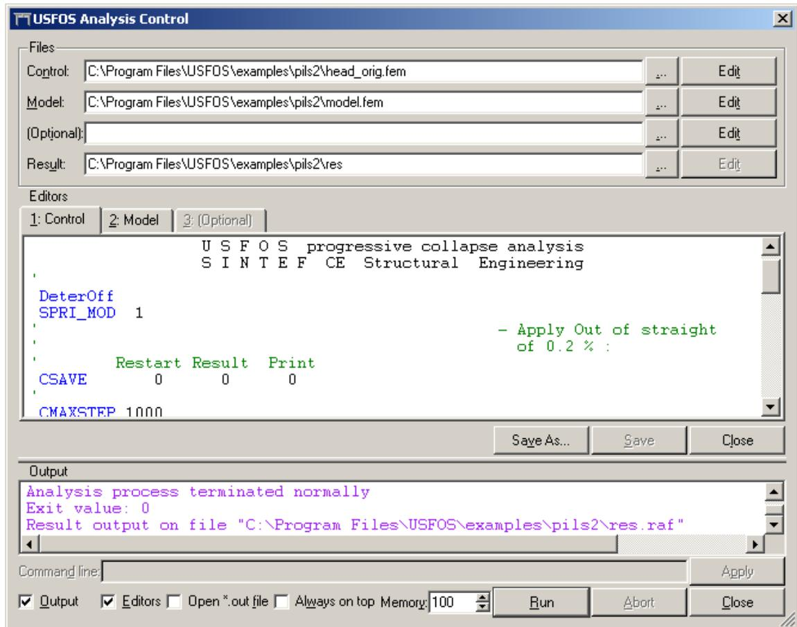
The upper part of the dialog contains edit controls where names of the input files and the result file should be given. They may be given manually or the corresponding browse buttons ([...]) may be clicked to bring up file dialogs for specification of file names. The name “res” will be suggested as name of the result file by default, which means that the results will be written to a file called “res.raf”.
