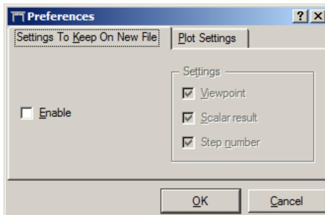
The “Plot Settings” tab has a check box that can enable usage of the size of the last plot that was created when a new plot is created:
