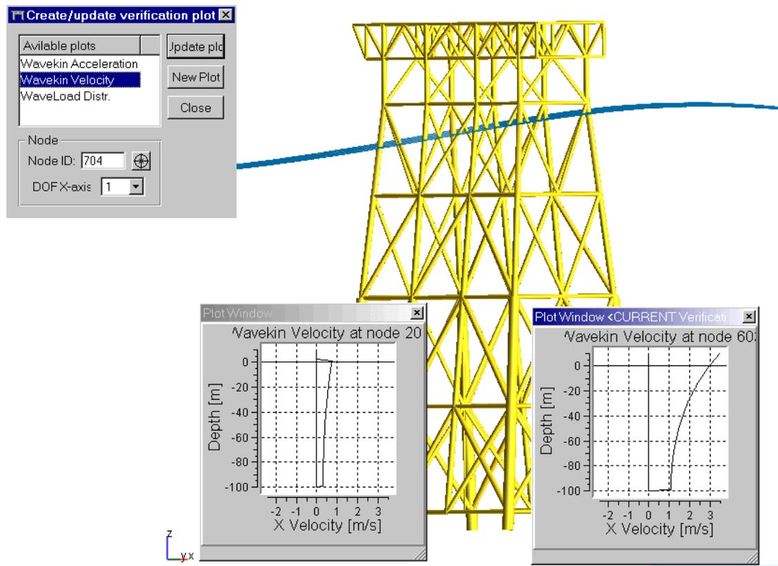
Figure 3.4-12 Plot of Wave Kinematics at different positions on the Jacket. .
