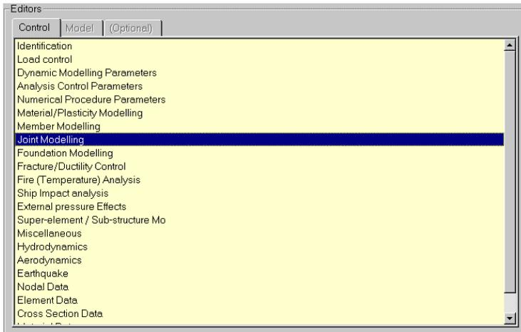
**Figure 3.3-12 Adding USFOS commands. Selection from the command menu, (F2 key)**
