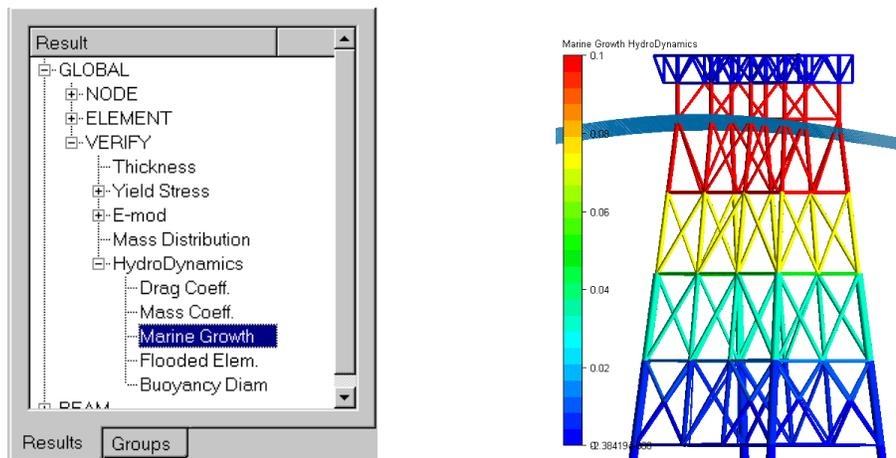
**Figure 3.4-1 Visualizing the Marine Growth on the individual members.**
