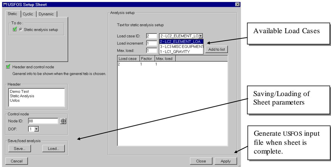
**Figure 3.3-7 Setup sheet for static analysis. Completed**
