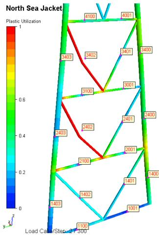
**Figure 3.4-6 Visualization of the utilization of one Row with element numbers applied.**
