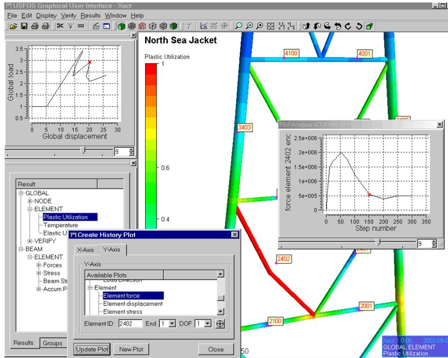
Figure 3.4-7 Visualization of the utilization of one Row with element numbers applied.
