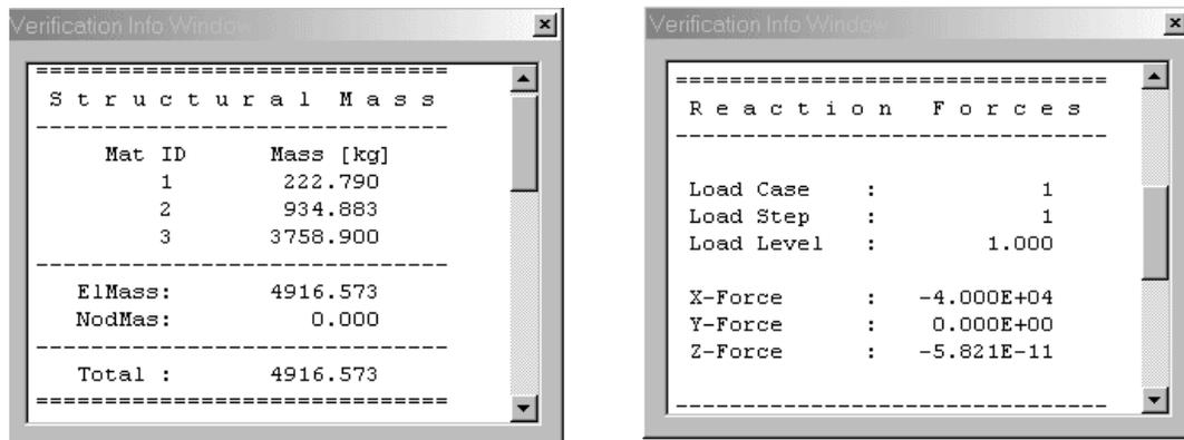
Figure 3.4-11 Print of Structural Mass and Reaction Forces .
