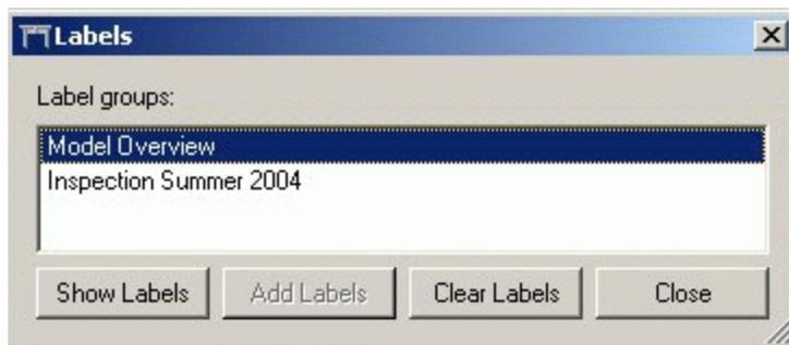
The dialog contains a list of the label group names. A label group is selected by pointing at its name and clicking it, or by using the arrow up/down buttons. “Show Labels” shows the selected group of labels. To show more than one group of labels simultaneously, click the “Add Labels” button. “Clear Labels” will remove all user-defined labels from the 3D view. The “Close” button closes the dialog.
