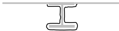
Figure 6-5 - Over side of top flange could be left open if documented sufficiently.
