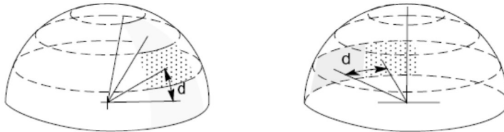
Figure 3-1 Ray-Tracing according to Shah and Lockwood.
